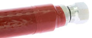
**Safe-Fire tape** (art. no SFS-TE3) is made of 100 % silicone rubber with heat resistance +260° C in continuous exposure. It is meant to seal the ends of fire sleeve and is available in
