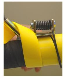
Start by rotating the spiral 1-2 rounds onto the hose / hose bundle (if the spiral is long it is better to start from the middle). Lift the spiral on top of the pin, the pin towards the mounting direction. Holding spring follows the hose. Turn the tool by its handle.
